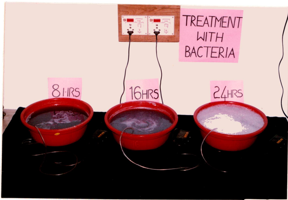
Fig. 5. Tannery effluent treated with bacteria for 8 Hrs, 16 Hrs and 24 Hrs.
