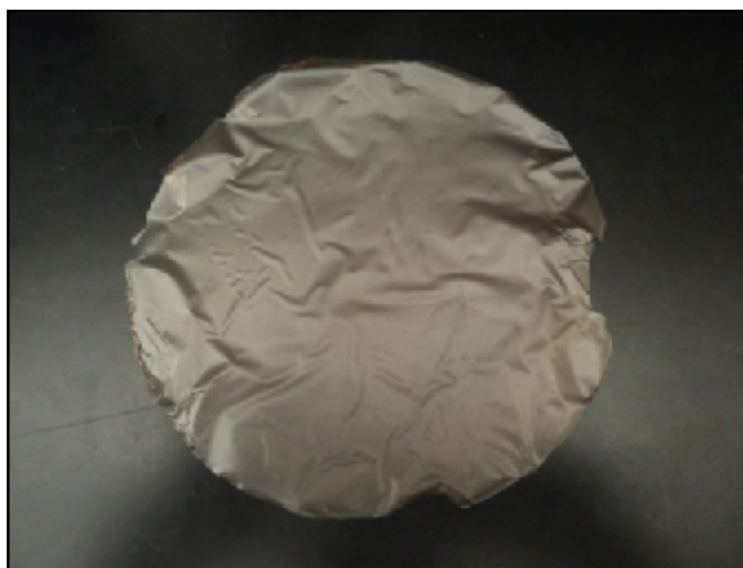
0.12 % Ag Nanoparticle Impregnated Edible Films
