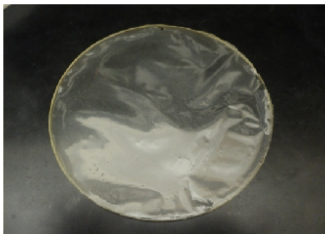
120 \mu l of Nanoparticle Impregnated Edible Films
