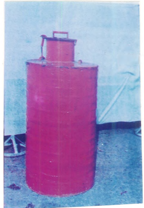
Plalte-IIId Coal-tar Drum Bin ->
