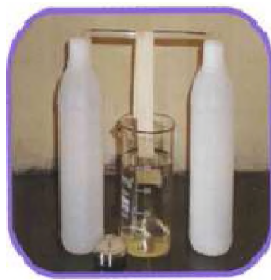
PLATE – XVI CAPILLARY RISE TEST
