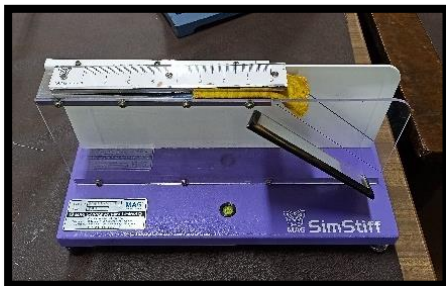
Plate XV Fabric Stiffness tester
