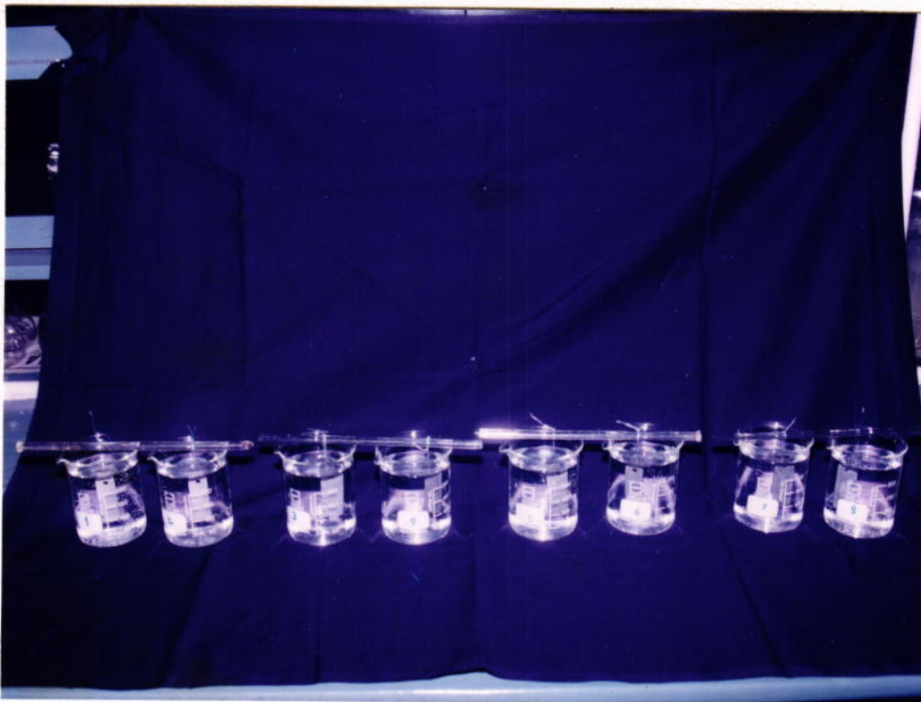
Photo-1 An experimental set up of weight loss method With hexadecylamine
