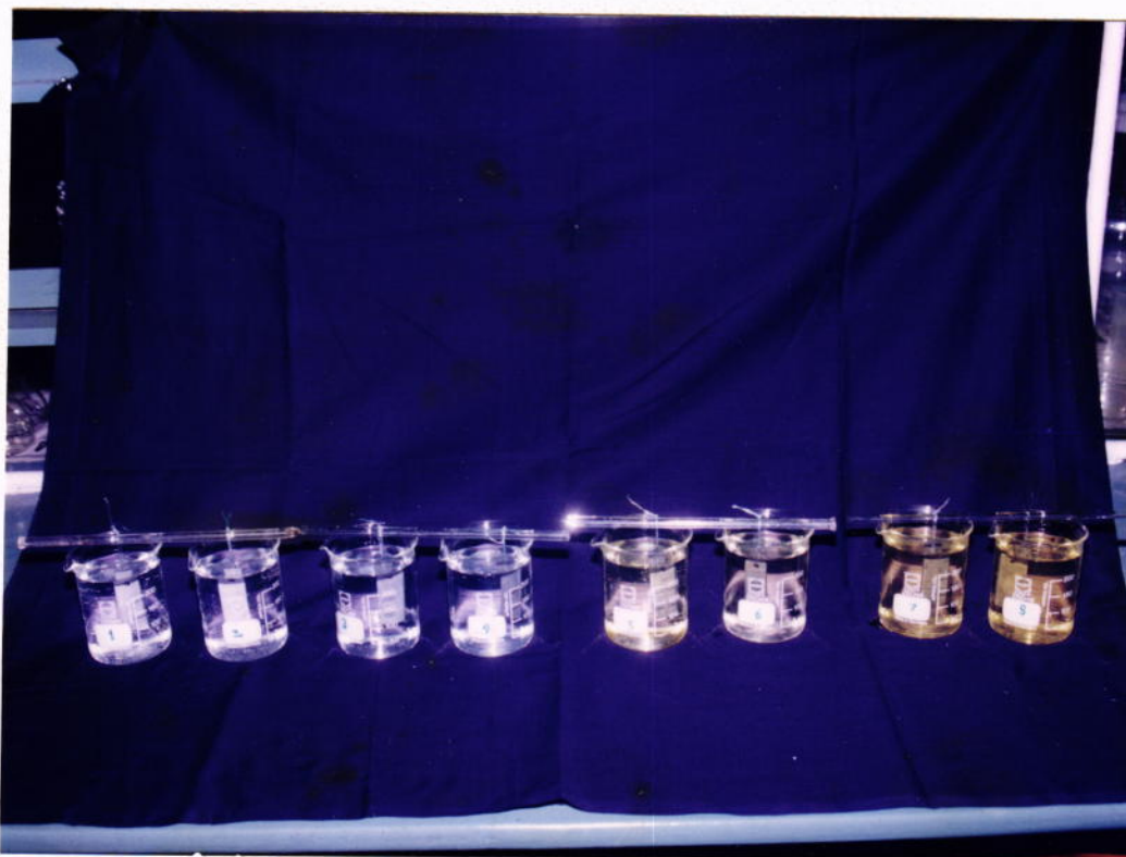
Photo-2 An experimental set up of weight loss method With hexadecylamine and halides
