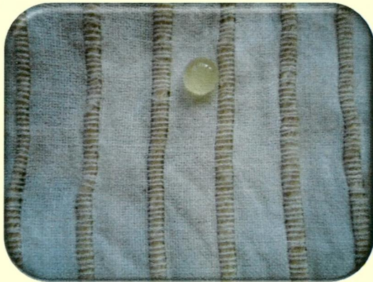
14a. Oil Drop on Treated Fabric
