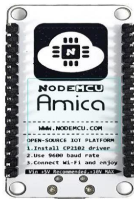
Plate - 3.6.1.2 (b) Node MCU used in Determining the Colour in the selected Recipes
