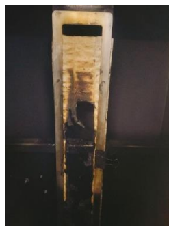
TS3 – Self extinguished
