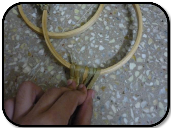
Plate VIII (b) Placement of fibre into the wooden ring
