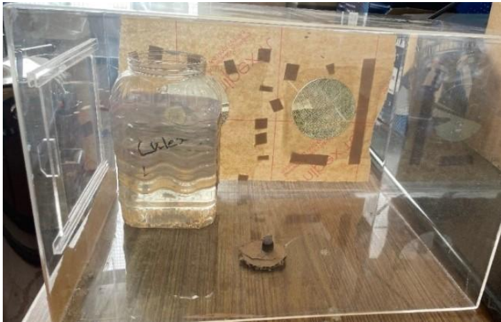
(C) - Vitex negundo incense bar mosquito repellent activity cage test
