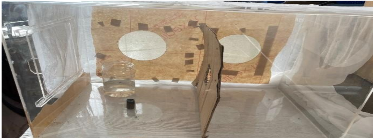
Figure: 22 - Efficacy of repellent in Excito – chambertest for Culex Spp. mosquitoes
