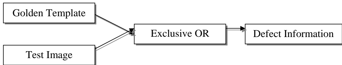
Figure 5.14 : XOR Based Image Subtraction for Defect Detection
