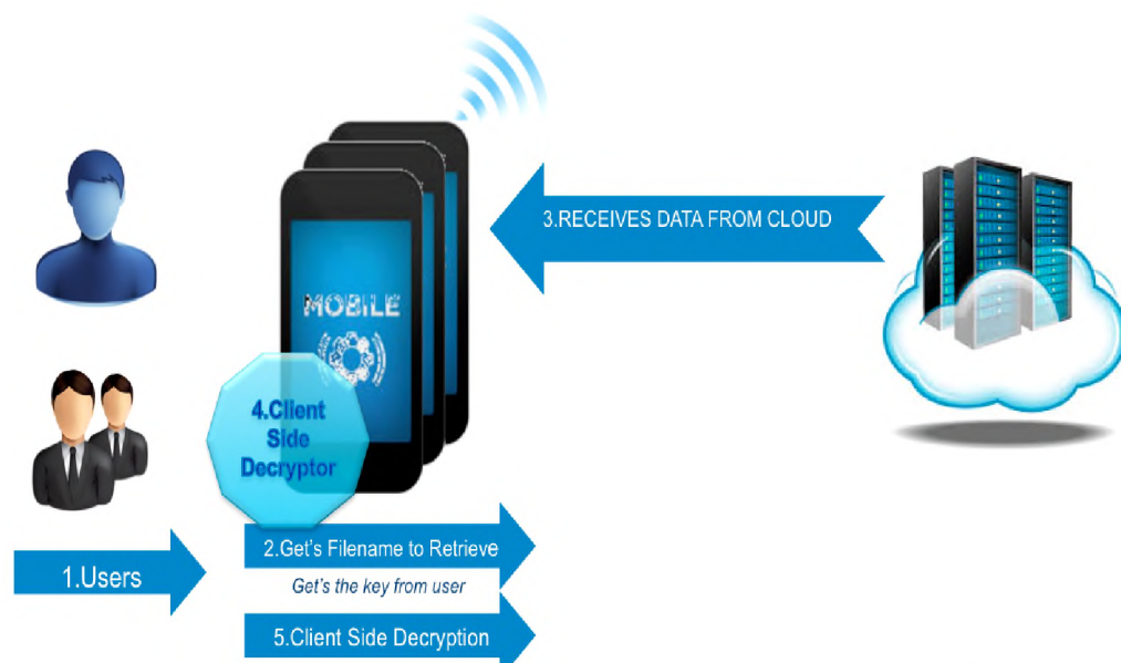
Figure 6.3 MSAES Decryption for Downloading Process
