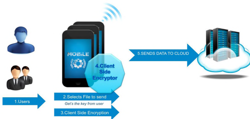
Figure 6.2 MSAES Encryption for Uploading Process
