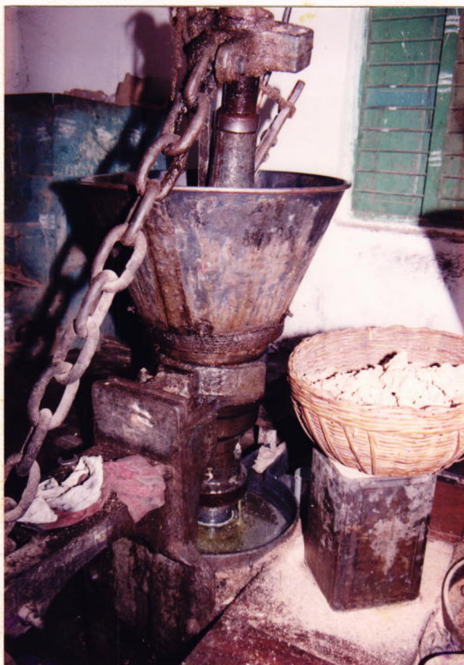
Plate I. Extraction of oil in the oil mill
