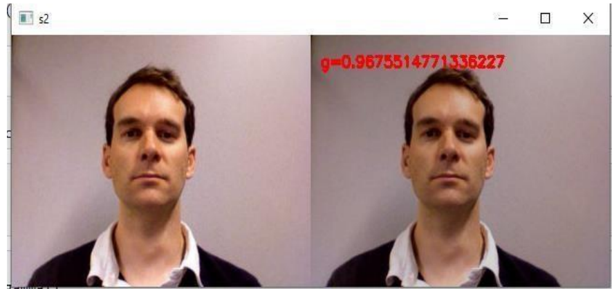
Figure 4.4: Before and after applying the Gamma Correction.
