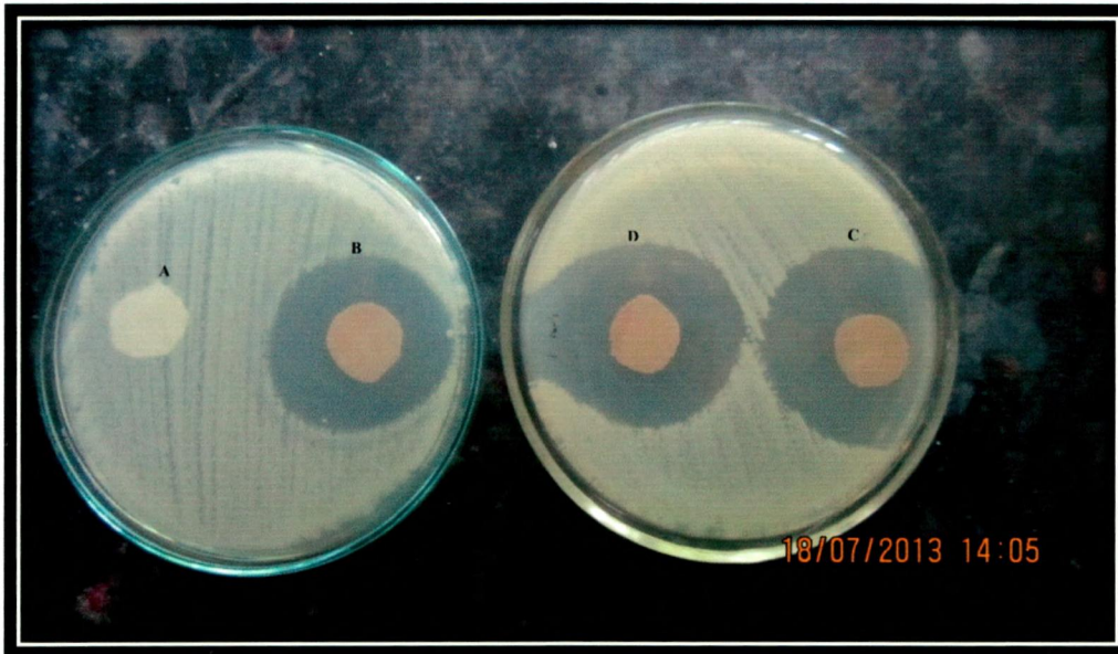
A - Control sample, B - Conventional sample, C - Ultra sonic atomized sample, D - Nano finished sampl
