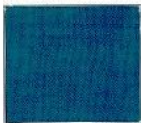
(SDS) Soft Water Dyed Sample Fabric - Cotton Weave - Plain Weave Dye Used - Direct Dye
