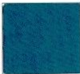
(BDS) Basic Dye Treated Water Dyed Sample Fabric - Cotton Weave - Plain Weave Dye Used - Direct Dye
