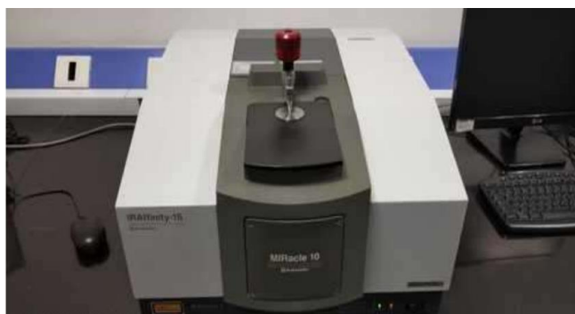
Image 10: FTIR Spectrometer (Miracle 10 SHIMADZU)
