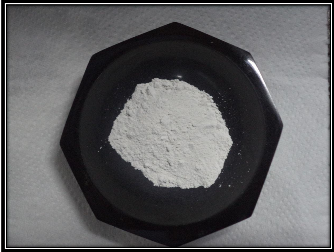
FIG 3.1, SYNTHESISED TITANIUM DIOXIDE POEDER USING HYDROTHERMALMETHOD
