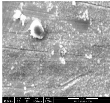
Figure 7. SEM images of brass (a) JBD and (b) CD in the experimental system
