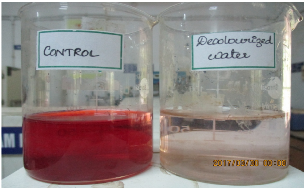
Control and decolourized solution of Acid Red 51
