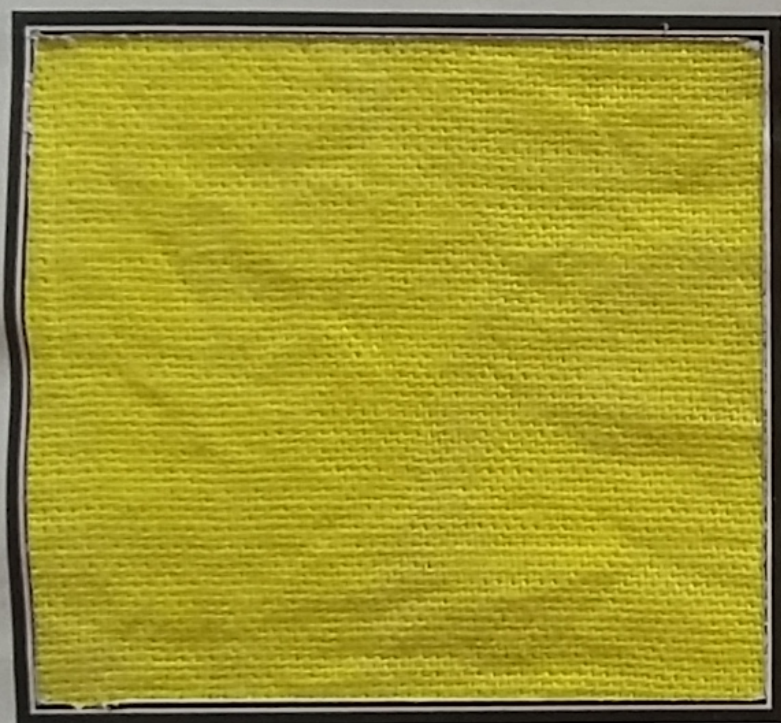
Fabric dyed with basic yellow 13 using fresh water
