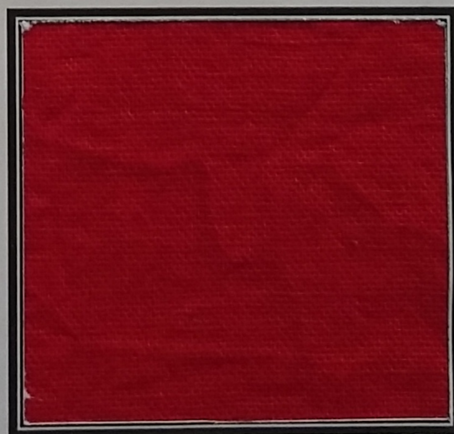
Fabric dyed with acid red 51 using decolourized water
