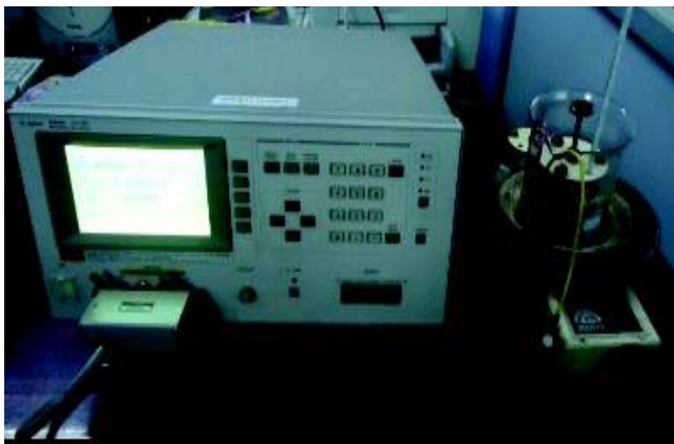
Figure 3.16: Experimental setup for electrical analysis (Agilent 4284A LCR meter)
