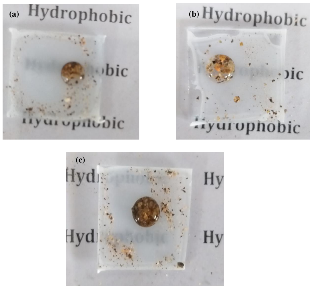
Fig. 4.54 (a) PDMS/PVDF, (b) PDMS/PMMA and (c) PDMS/PS coated substrates showing Self cleaning property.
