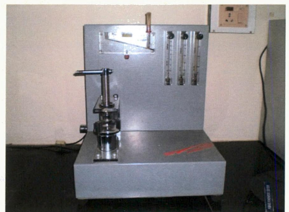
Plate – 35 Shirley Electronic Air Permeability Tester
