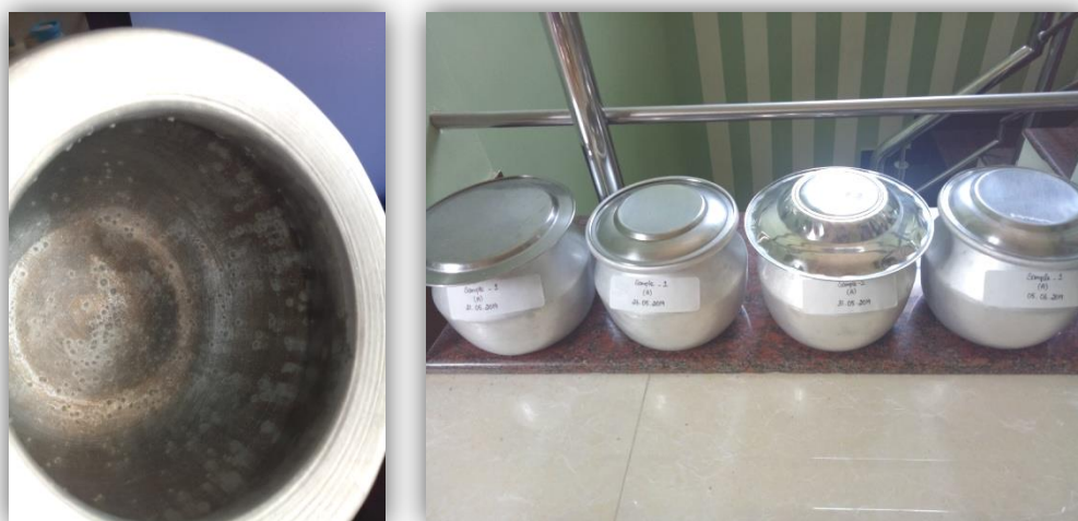
Plate 11: Pitting in Aluminium Container Storage of Water in Aluminium Containers
