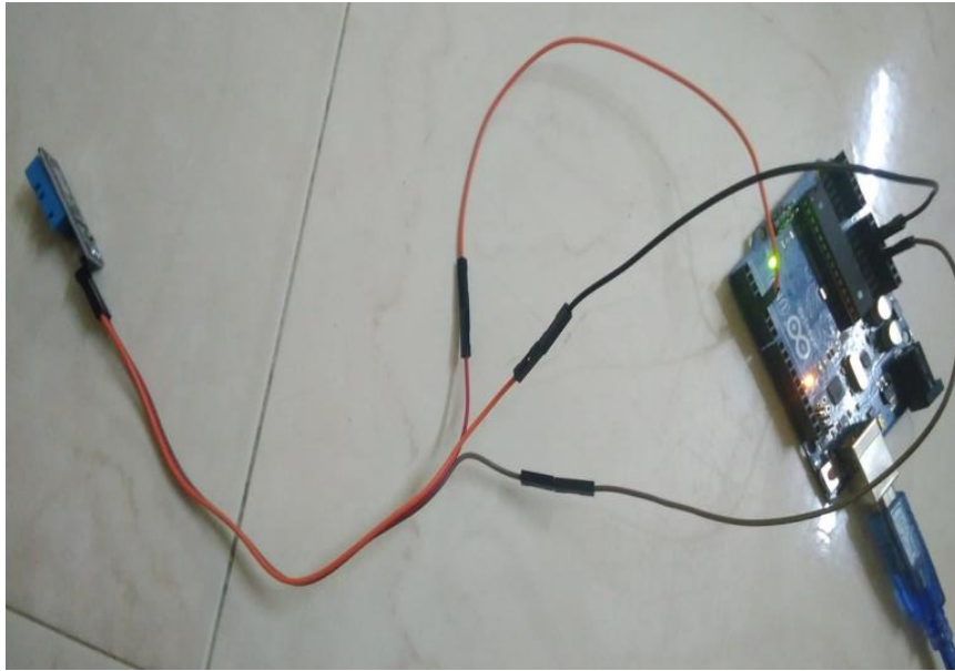
Fig 9.7. DHT11 sensor connection with Arduino
