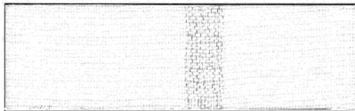
CI (5 cm cotton yarns with 1 cm copper conductive yarns)
