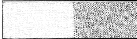
AG (5 cm cotton yarns with 5 cm aluminium conductive yarns)
