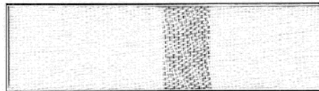
AI (5 cm cotton yarns with 1 cm aluminium conductive yarns)
