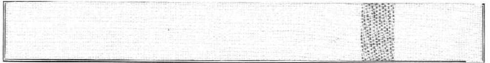
AC (15 cm cotton yarns with 1 cm aluminium conductive yarns)
