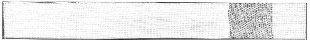
AB (15 cm cotton yarns with 2 cm aluminium conductive yarns)
