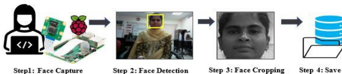
Figure 5.7 Framework for Facial Expression Dataset Collection using IoT Kit
