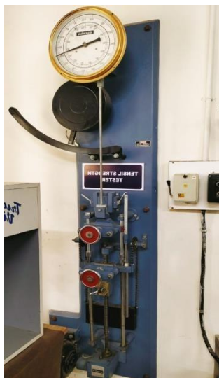
Plate – 8 Tensile Strength Tester
