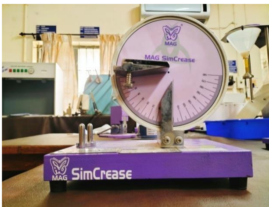
Plate- 10 Crease Recovery Tester
