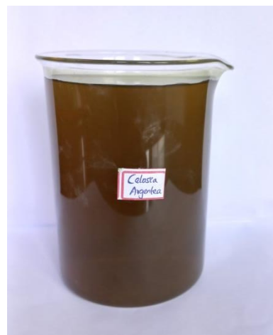
Synthesized silver nanoparticles of Celosia argentea
