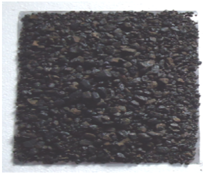
Fig (4.1) Photographic view of tar coated blue metal
