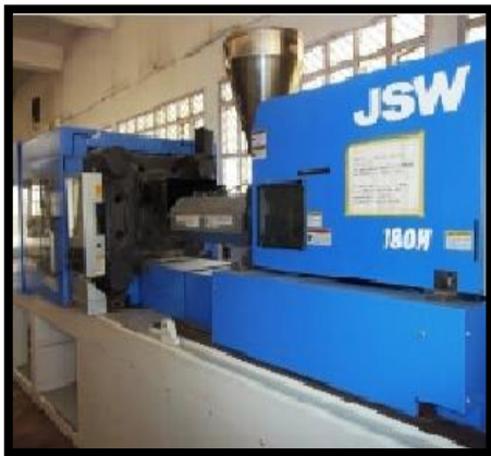
Plate-XV Injection molding machine
