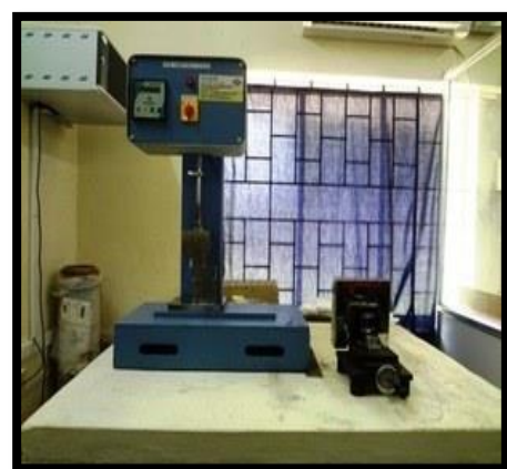
Plate-XVIII Charpy Impact strength tester
