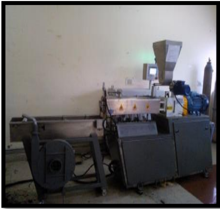
Plate-XIII Twin screw extruder
