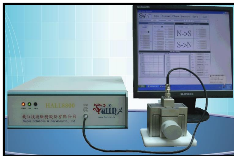
Figure 3.5 Hall Effect Measurement System
