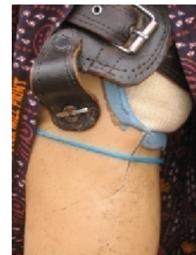
Figure: 40 Broken Socket
