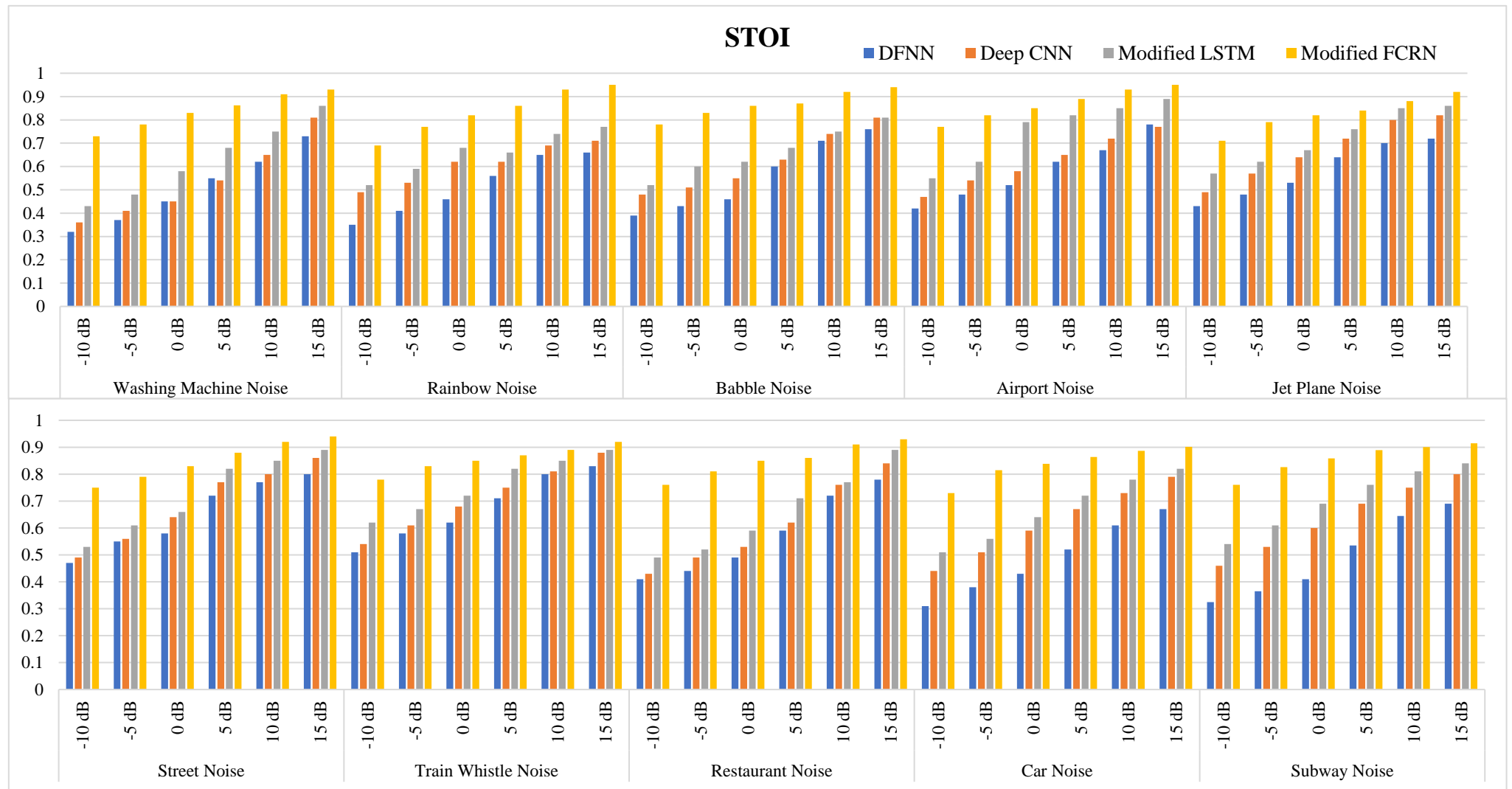
Figure 6.5 Comparative Analysis of STOI of DNN Algorithms for Alaryngeal Speech at Various Noise Types and Levels
