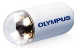
Figure 1.2 Wireless Capsule Endoscopy ( https://www.olympus-europa.com )
