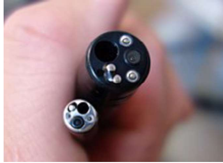
Figure 1.4 Insertion Tip of a Typical Endoscope ( https://en.wikipedia.org/wiki/Endoscope )
