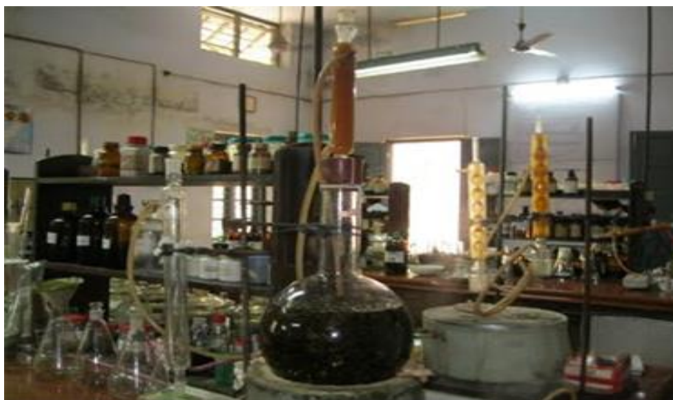
Fig.4. Soxhlet apparatus used for plant extraction
