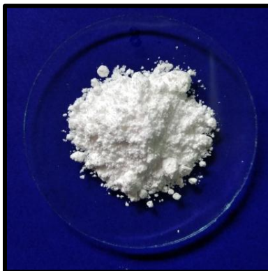
Figure .3.3.1 (a) Ni-BDC Metal Organic Frame work (Powder form)
