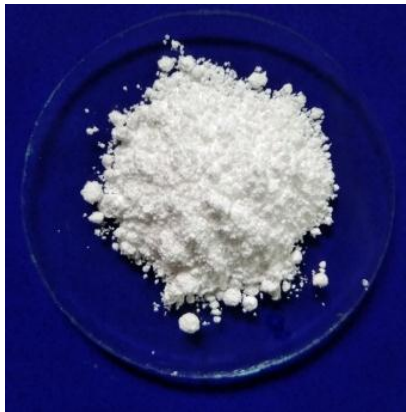
Figure .3.3.1 (f) Al-BDC Metal Organic Frame work (Powder form)
