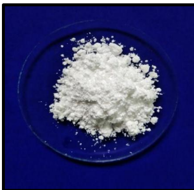
Figure .3.3.1 (e) Zr-BDC Metal Organic Frame work (Powder form)
