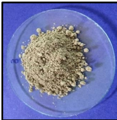
Figure .3.3.1 (b) Cu-BDC Metal Organic Frame work (Powder form)
