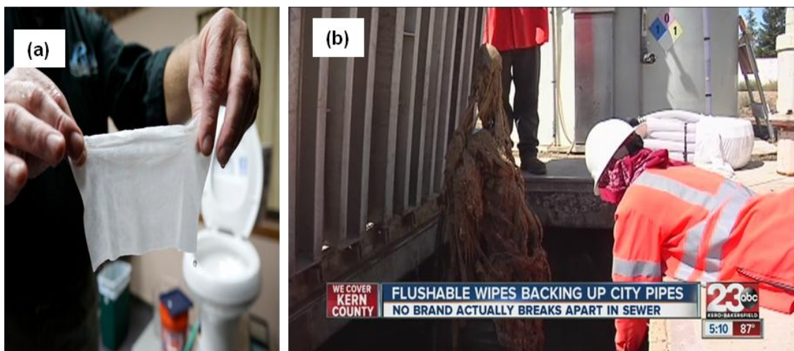
Images of (a) flushable wipes and (b) a screen shot of an video file, showing the rescuer in action of removing the sewage block caused by flushable wipes in Bakersfield city, (California)
