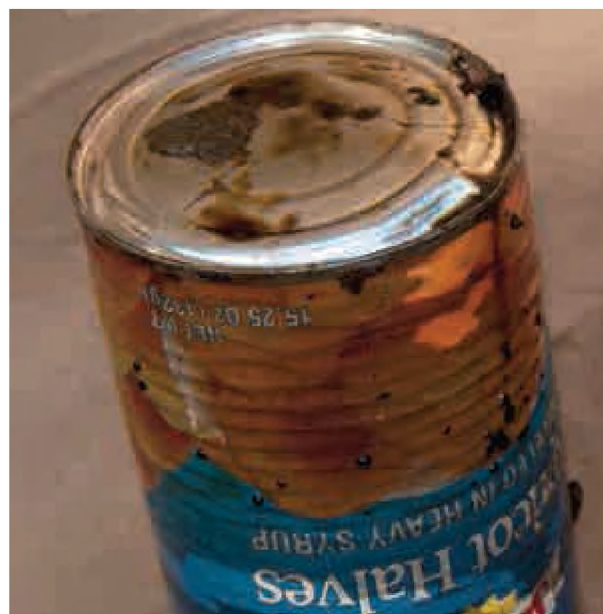
▲ Plate 8.11 Sign of Leakage
