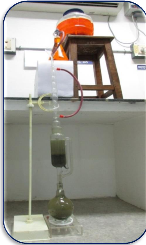
Plate 10 - Column study for methyl orange decolourisation at lab scale
