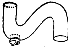
FIG. 62 S-bend with screw
