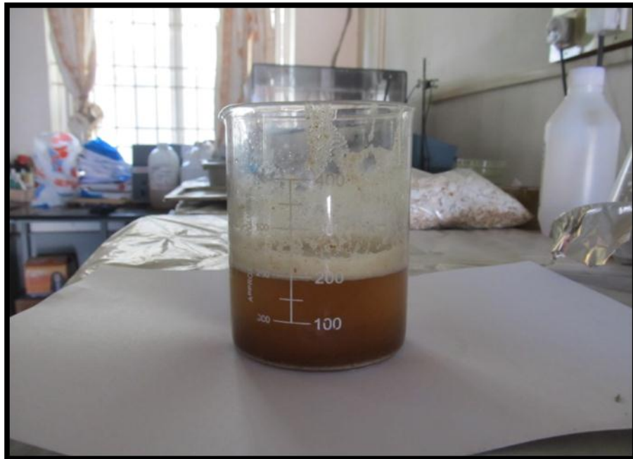
PLATE 3 WASHING THE POWDER WITH ACETIC ACID
