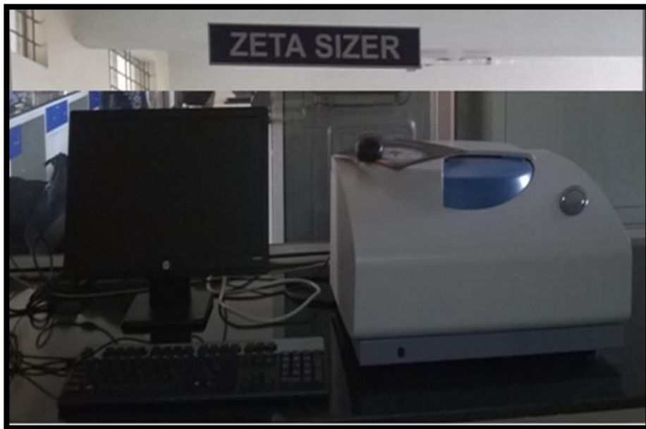
PLATE 11 PARTICLE SIZE AND ZETA POTENTIAL ANALYSER
