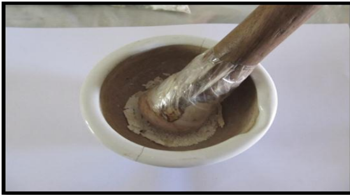
CRUSHING OF EGGSHELL POWDER
