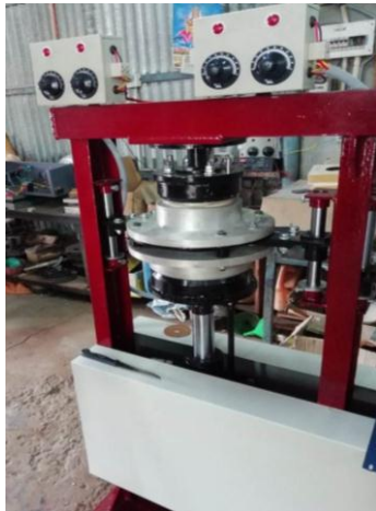
Hydraulic press was applied with the application of 1.5 ton of weight
