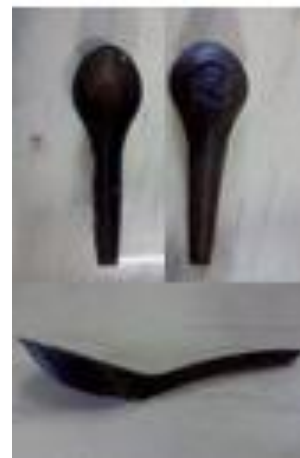
Edible cutlery made using Hydraulic pressure method
