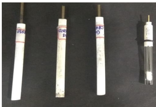
Figure 10. Fabricated carbon paste electrode and Standard glassy carbon electrode
