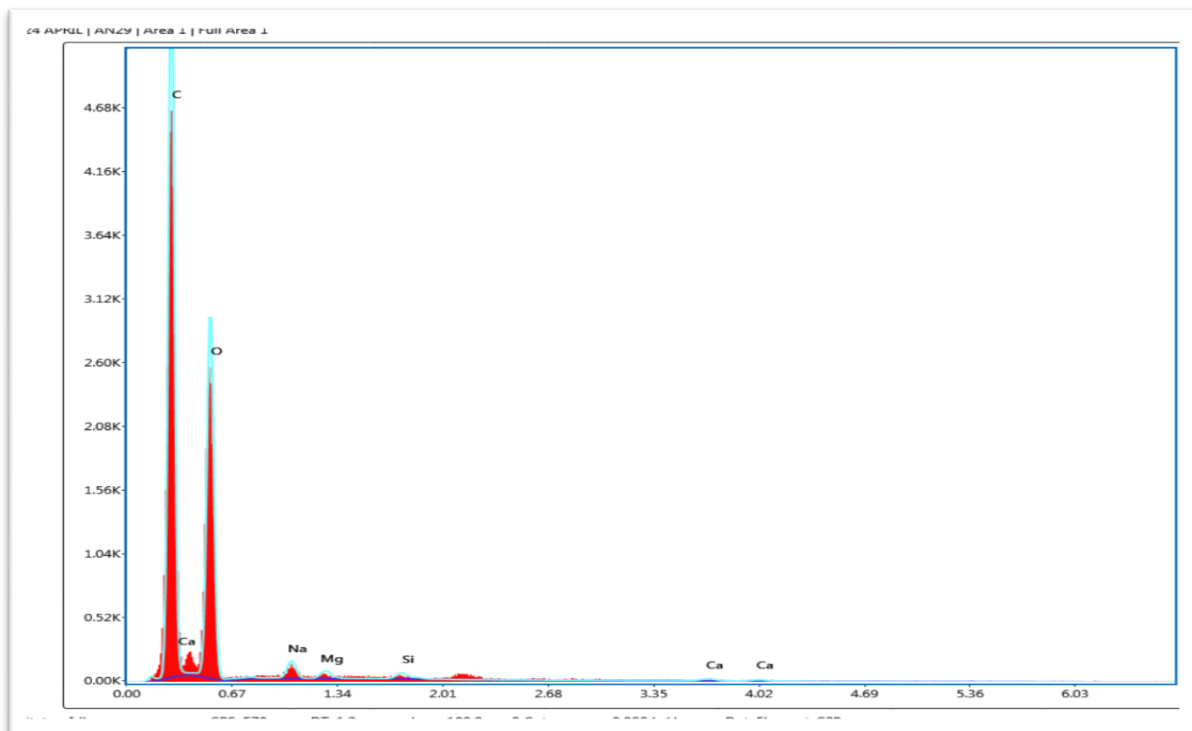
Figure 14: Elements present in the C-G-PVA silver nanoparticles of T. procumbens composite film analyzed by SEM
