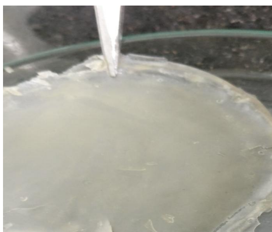
Fig 15 e. Solid polymer film of PGMCSN7
