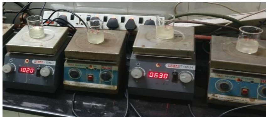
Fig 15 b. stirring for 24 hours in a magnetic stirrer (Group)
