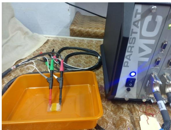
Fig 21 b. Thin film probe set up
