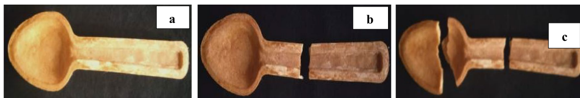
Fig. 5 Drop test of sorghum spoon. a 40 cm of SRS, b 50 cm of SRRS, c 50 cm of SRHS
