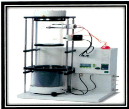
PLATE - X NANO SPRAY DRIER
