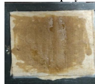
Plate 6f Pouring resin on reinforcement fabric
