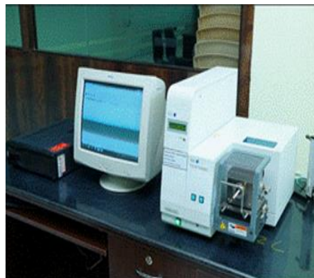
Plate 3b Thermogravimetric analyser
